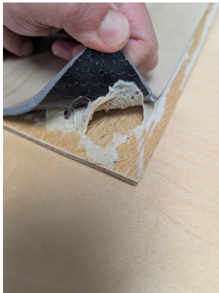
Figure A5 — Adhesive / Flooring Interface
